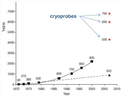
$$\frac{S}{R} = K \frac{N^2 V^{3/2}}{T_s} \sqrt{\frac{C_f Q_p V_s}{T_p^2 T_R}}$$
